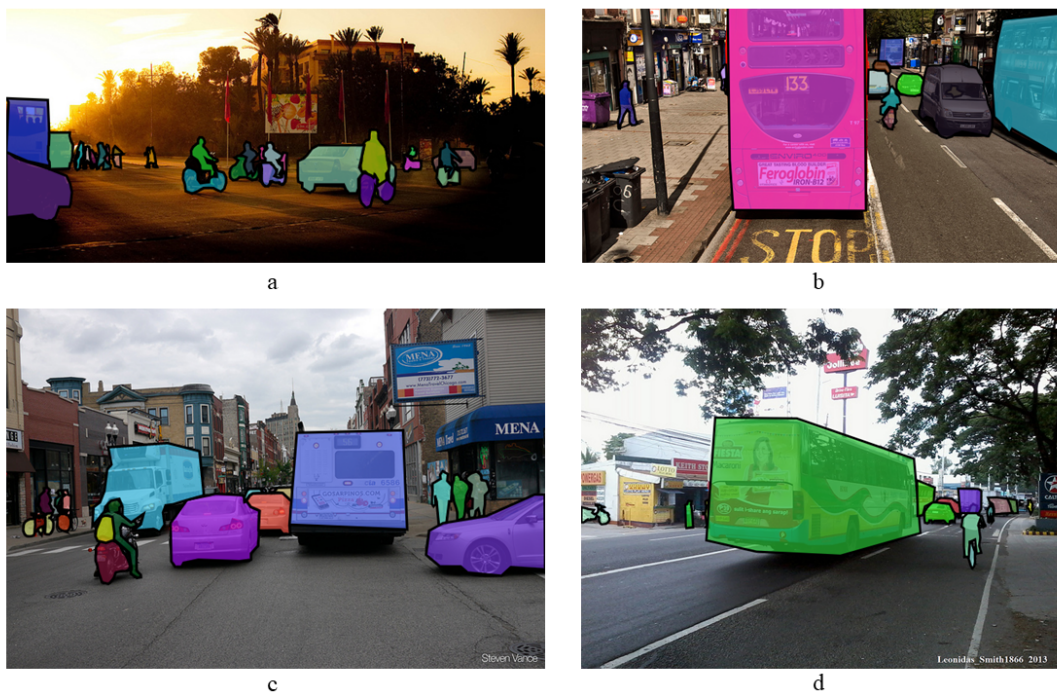
Fig. 4. a,c,b,d are a sample of vehicle detection images found in the COCO dataset. The coloured shapes mask the edge of the vehicles. This is used both for training as well as testing to measure the accuracy of the detection model.
